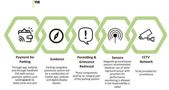
» Figure 4: Components of the smart parking solution in Panaji (IUC 2021)
