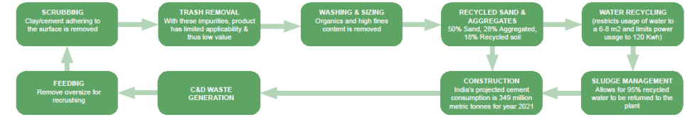
Figure 5: Circular model adapted for C&D waste recycling at Surat, India
